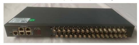
Ethernet with a fast protection based on E1 events. This jumps of parallel E1's are generally microwave radio or G.SHDSL in parallel.
