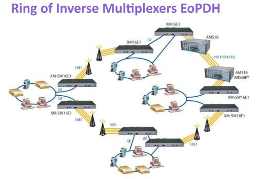
The **XM-SW16E1-4TTX** is particularly interesting to deploy a Ethernet ring over E1 microwave radio, DSL coppers. Typically the transport domain must deploy secure Ethernet infrastructure over existing E1 infrastructure.
