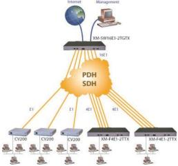
The *XM-SW16E1-4TTX* is a switch of E1 carrying Ethernet over TDM EoPDH.
