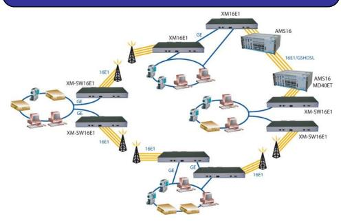
The **XM-SW16E1-47TX** is particularly interesting to deploy a Ethernet ring over E1 microwave radio, DSL coppers. Typically the transport domain must deploy secure Ethernet infrastructure over existing E1 infrastructure.
