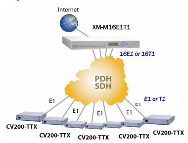
The **XM-M16E1T1-4TTX** can tag or double tag the incoming traffic from the Ethernet or from the E1 or T1 WAN.
