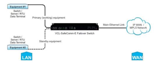
Equipment 1 fails. Ethernet link automatically switches to Routers, Servers, Switches, RTUs, Data Terminals (any terminal) etc.
