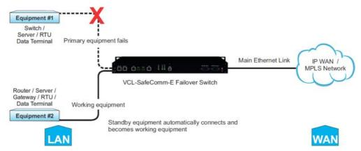
Equipment 1 recovers. Ethernet link automatically reverts and reconnects to Routers, Servers, Switches, RTUs, Data Terminals (any terminal) etc.
