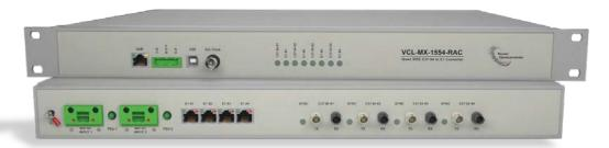
VCL-MX-1554-RAC, Quad (4x) IEEE C37.94 to E1 Converter is a ruggedized and robust, sub-station-hardened protocol converter that converts up to 4 x IEEE C37.94 Interfaces to 4 x 2.048Mbps E1 and vice-versa. The VCL-MX-1554-RAC, IEEE C37.94 to E1 Converter supports point-to-point as well as point-to-multipoint applications. Designed for inter-connecting IEEE C37.94 Differential Protection Relays over and E1/SDH network.
