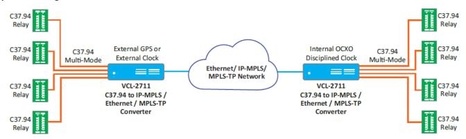
By installing the VCL-2711, the existing C37.94 Protection Relays can be migrated from an SDH / SONET transmission network to an Ethernet / MPLS-TP / IP-MPLS transmission network with no degradation or compromise in the reliability or the performance of the C37.94 interfaces.
