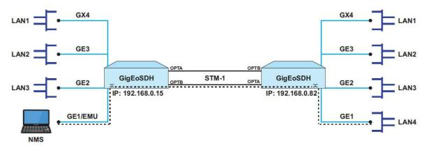
Note: Make sure optical A of one NE must be connected with optical B of its neighbouring NE.
