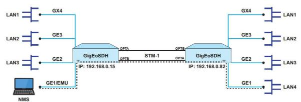
Note: Make sure optical A of one NE must be connected with optical B of its neighbouring NE.
