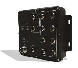
SWMH-3110-PM series are a ruggedized switching platform that complies with the most demanding IP67 industrial standards, designed for industrial applications requiring completely potted to protect against water, shock and vibration. SWMH-3110-PM series provides 8 Fast Ethernet M12 PoE ports and 2 Giga Cooper interfaces. With the managed features, users are easily to prioritize, partition and organize user's network and provide reliable and high quality services.
