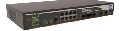
**SWCE-3400** enables Carrier Ethernet 2.0 and IP connectivity services. including EVC, E-LINE / E-LAN / E-TREE at a UNI / NNI Carrier Ethernet network access.
