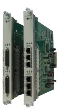
DCE interface are supporting RS232 but we can supply this interfaces card with X21/DB15F Synch cable adapter or with RS422/DB25F or DB9F adapters.
