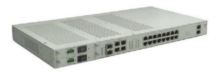
The CXR HX9150 SDH STM1 TM/ADM is a standard equipment device for SDH/MSTP networks with VC-12 directly reaching the network terminal. Through an STM-1 uplink, the HX9150 provides VC-12 standard E1s and Ethernet supporting VCAT, GFP, and LCAS protocol.
