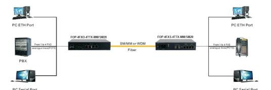
In private networks, Optical Multiplexer shares services such as FXS/FXO, RS232/RS485, Ethernet, in P2P topologies over fiber. 4FXS/FXO Optical Multioplexer establishes TDM and Ethernet connectivity between the remote branches and headquarters for edcational, financial and military sectors.
