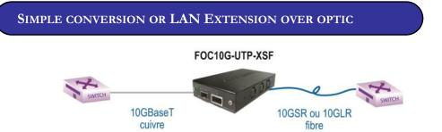
The FOC10G converters supply the interconnexion of 2 x 10 Gigabit/Ethernet copper or fiber of any vendor according to IEEE 802.3an/.3ak/3ae. The adapting function of copper port are fully automatic and LED are giving information on traffic.
