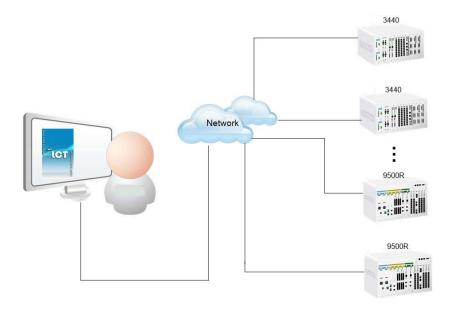
CXR-iNET-LCT is able to manage only one by one node.
