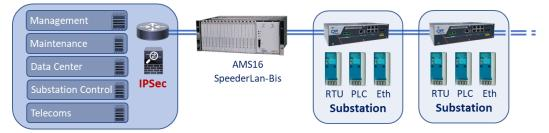
CopperWay-Bis-HV3 connects all the equipment of the 20 KV substation over a communication infrastructure made of pilot cables and fiber optic cables to the data center. It delivers many Ethernet ports to connect all substation systems. It embeds very strong security features to secure the substation communications including IPSec, X509 authentication and a hardware secure element.
