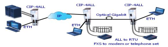
The Circuit Emulation over Packet processor delivers high performance, extremely low latency, and a perfect distortion-free transport of the analog signals. The CIP-ALL provides many emulation protocols and a dual 10/100 BaseT and optical Gigabit Ethernet connectivity to adapt to any network requirement.
