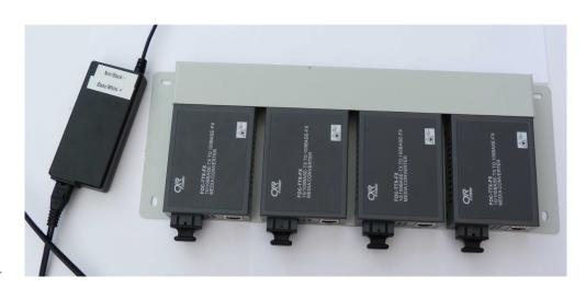
The **Q-FOC** kit is a black or grey metal part with AC/DC converter witch provide **a four independent media converters** on compact form and with the possibility to fix them on the wall or under the table in order to protect the fiber.
